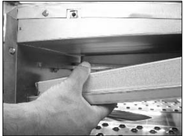
13. Lower the end of the finger assembly.
